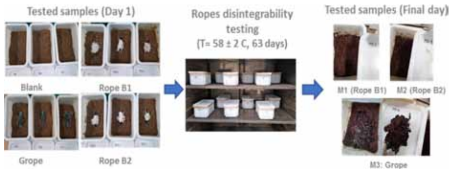
Figure 3. Disintegrability test in simulated lab composting conditions. BIOGEARS (B1&B2) vs. GROPE (ref.).
